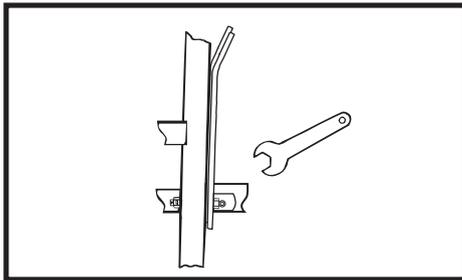
**3** **⚠️ WARNING:** Do not stand on the access ladder during this procedure! The person who performs this procedure must be standing on the floor or a stepladder. Remove the nut and carriage bolt that connects the mechanism to the rail of the ladder. Discard the old carriage bolt and lock nut.
