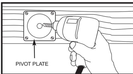
**6** After checking for squareness and straightness drill a 13/64" diameter pilot hole into the access ladder frame and the rafter using the pivot plate as a guide. Make sure the drill is
