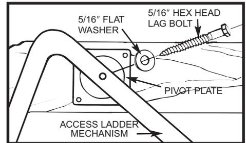
The lag bolt must be perpendicular to the frame. Tighten the lag bolt until the mechanism is firmly against the pivot plate. The mechanism should be easily moved by hand without any gap between the mechanism and pivot plate.
