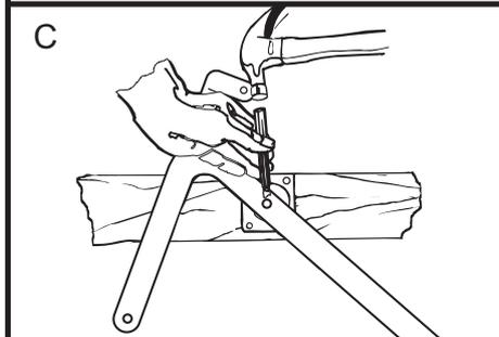
horizontal and perpendicular with the frame. It may be necessary to push the rivet out of the way so that the hole is clear to drill. The rivet will remain in the pivot plate and will not interfere with drilling or the function of the access ladder.
